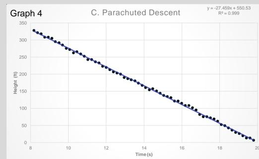
Graphs 2, 3, & 4 give a closer look at each part of the rocket's flight. Both parts of the ascent could be modeled by parabolic equations while the parachutes descent is fitted by a linear equation.
