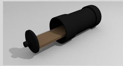
To secure this section of the rocket and prevent damage to the hardware, the payload bay was constructed using polyvinyl chloride (PVC), a rigid plastic. In addition, the Arduino and altimeter were secured to the electronics bed using plastic screws. The hardware bay was mounted within the payload tube, which also served as the coupler tube seen in the diagram below.
