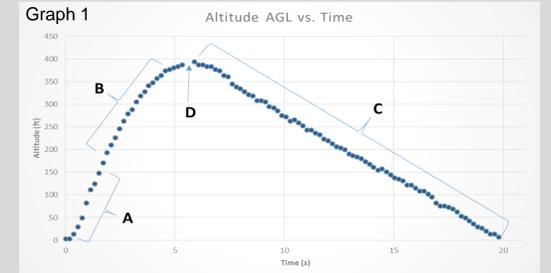
Graph 1 shows the altitude of the rocket for the complete flight, including the powered ascent (A), coasting ascent (B), apogee (D), and the parachuted descent (C). AGL is an acronym for above ground level.
