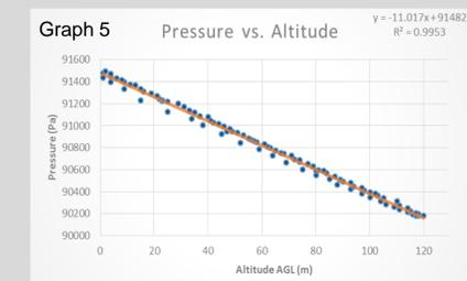
Graph 5 demonstrates the inverse relationship between altitude and atmospheric pressure. AGL stands for above ground level.
