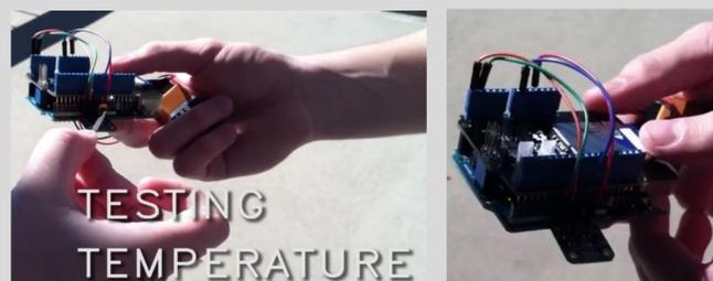
A match is used (right) to briefly increase temperature near the BMP sensor. An SD card (left) is used to collect pressure, temperature, and altitude data from the Arduino.
