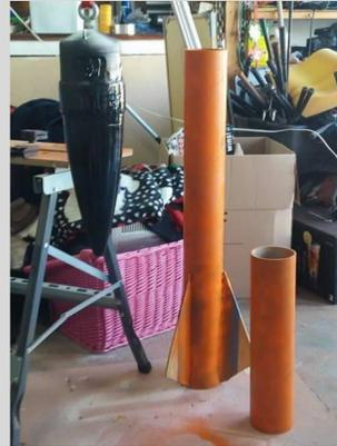
The body tube of the rocket was constructed using recycled materials. Plywood was used to construct the fins, bulk plate, and electronics bed. The data collection hardware, which included the Arduino, BMP sensor, and recovery altimeter (RRC2+), was housed on the hardware bay within the payload section.
